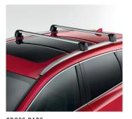
CROSS BARS These cross bars comply with Honda's stringent safety requirements. They need to be combined with roof rails and have a maximum carrying capacity of 75kg.
