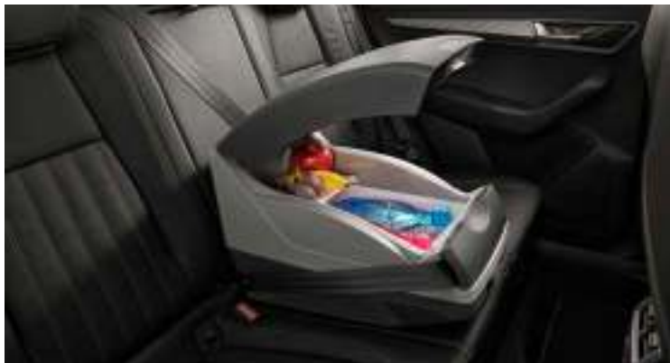
Thermoelectric cooling/warming box (15L) (5L0 065 400)
